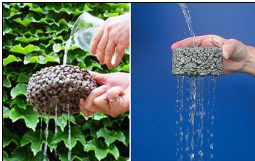
Figure 6. illustrative permeability of concrete Source: Ecodevelopment, 2009
