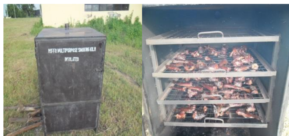
Figure 3. Showing the smoking kiln and smoking process
